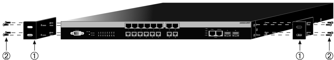
Figure 2-2 Attaching the Rackmount Brackets
